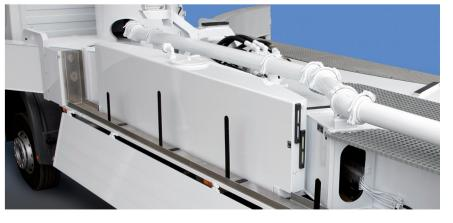
The torsion resistant frame that transfers the outrigger forces directly to the corner points provides enough space for a 600l oil tank and room for hoses and pipes.
