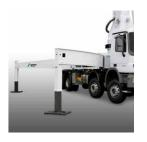
by SCHWING combines high torsional rigidity and excellent stability with minimum space requirement. The protected piston rod and internally laid hydraulic cables prevent damage and reduce service costs.
