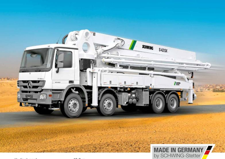
$\begin{tabular}{lll} Vertical reach & 42.2 m \\ Concrete output & max. & 162 m^3/h \\ Pressure on concrete & max. & 85 bar \\ \end{tabular}$
