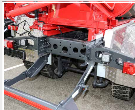
LED auxiliary headlights at the rear (2 pieces)
