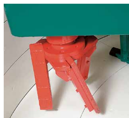
Agitators with reinforced agitating tools experience particularly low wear.
