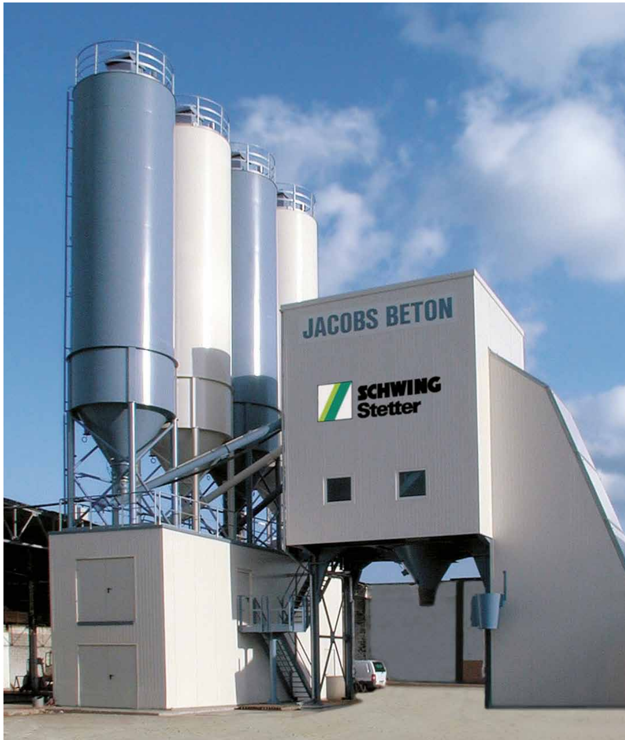
HN 3.0 with twin-shaft mixer, capacity 127 m 3 /h compacted concrete.
