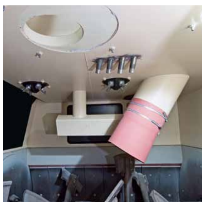
Nozzle heads for cleaning of the mixer.
