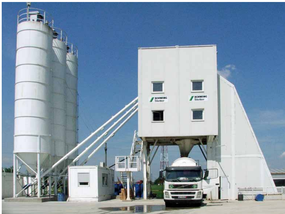
HN 2.25 with pan mixer, capacity 108 m 3 /h compacted concrete.
