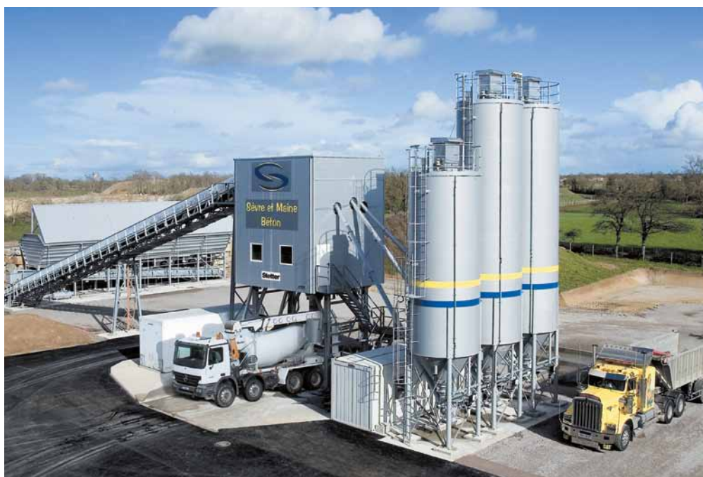
HN 1.5 with pan mixer, capacity 80 m 3 /h compacted concrete.
