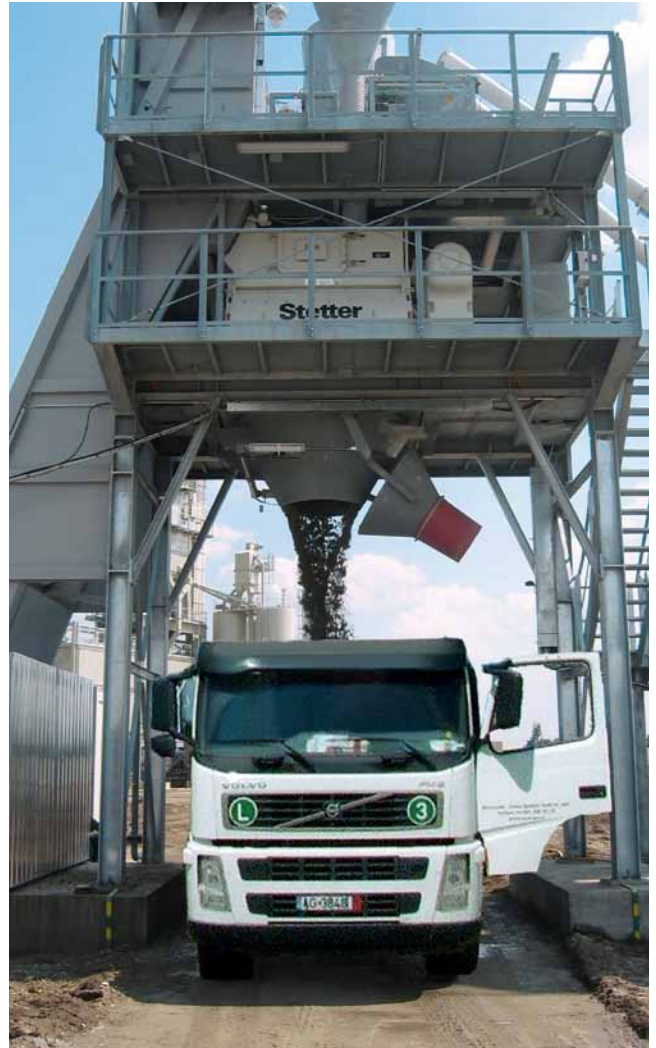
Discharge onto open truck.
