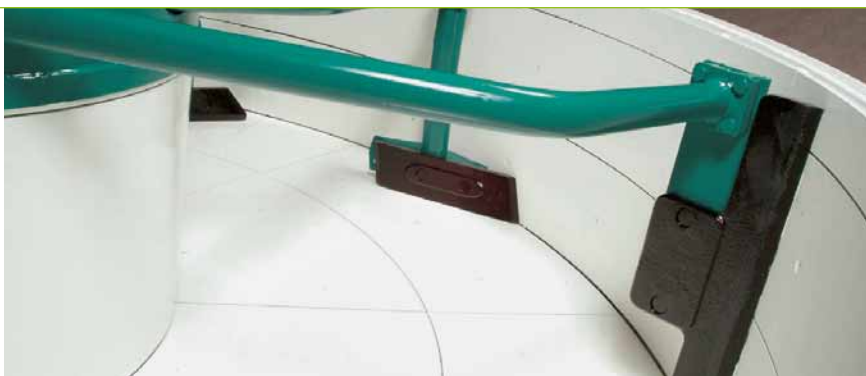
Pictures top left and right: the inner and outer scraper support mixing and discharging effect.
