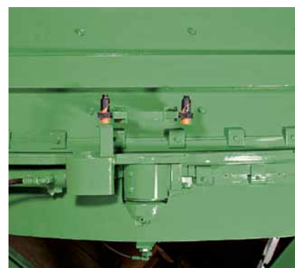
Power failure? Taking this into account, we have integrated a hydraulically operated manual discharge device.
