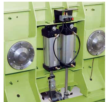
The pneumatic discharge gate operation.
