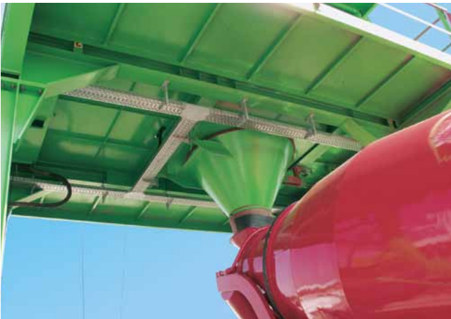
The mixer discharge for filling truck mixers.
