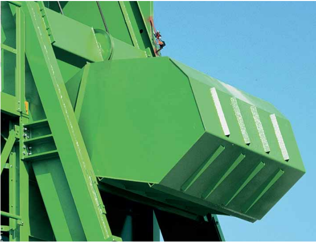
The large-dimensioned skip with an optimum shape guarantees complete emptying.
