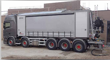
Machines from the BreMAT F-series can also be mounted on a truck chassis.
