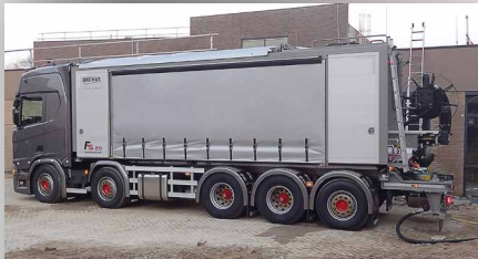
The BreMAT F4.15 consists of a 4-axle truck chassis and the F5.17 is assembled on a 5-axle truck chassis.
