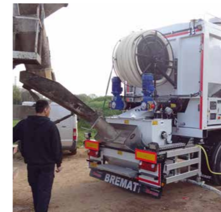
Raw materials can be added without interrupting the production process
