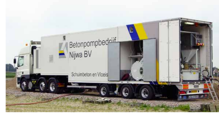
A foam mortar is produced on the basis of dry materials. The stock is kept in internal or external silos.
