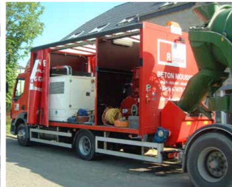
Truck mixers supply base mortar, which the machine foams and pumps.
