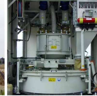
A foam mortar is produced on the basis of dry materials. The stock is kept in internal or external silos.
