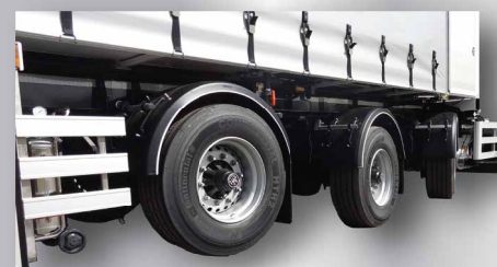
For a perfect turning radius and optimal weight distribution, the widespread semitrailer chassis consists of three 10-ton axles, including two steering axles.
