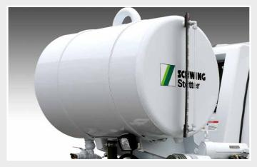
The large water tank for the CP 1800 D and the CP 2800 D has a volume of 450 litres and allows the machine and hoses to be thoroughly cleaned after completion of concrete paving.
