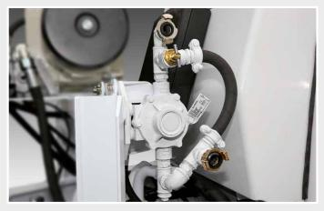
Once the concreting work is finished, the water pump facilitates cleaning of the CP 1800 D / CP 2800 D with up to 80 l/min and up to 20 bar of water pressure.
