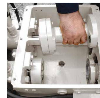
7 Lubricate delivery piston all around and retract into delivery cylinder
