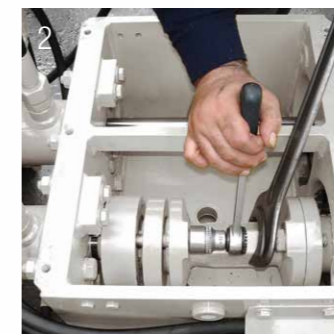
2 Release the screw connection of the adapter piece
