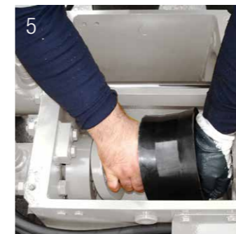
5 Remove used delivery piston, insert new delivery piston
