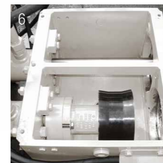
6 Lubricate delivery piston all around and retract into delivery cylinder
