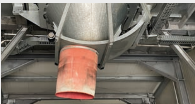
Lowerable discharge funnel with drip protection
