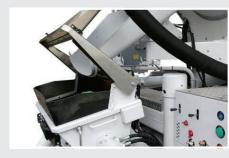
Covering for hopper in position "Own + external filling"
