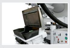
Covering for hopper in position "External filling"
