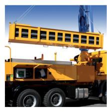
The hose storage boxes on the right side can be loaded and unloaded by a fork lift, crane or the pumps own boom.
