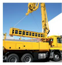
Additional storage boxes for hoses and pipes can be loaded and unloaded by fork lift, crane or the pumps own boom to place them where they are needed.
