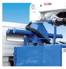
2 slewing cylinders on each side of the turret guarantee safe and dependable operation.
