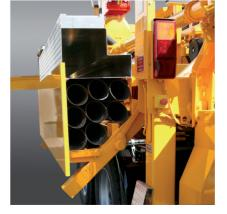
The hydraulic hose box can be lowered without outriggers down and putting the hoses within easy reach of the operator.
