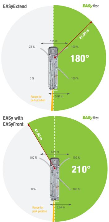
The outrigger spreads as specified are measured from the centre of the outrigger leg. Any cribbing or underlay timbers must be taken into account when determining the required set-up area.
