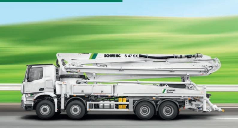
Vertical reach46.10 mConcrete outputmax.162 m³/hPressure on concretemax.85 barTare weightapprox. 31 t
