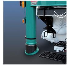
Operator friendly - the swivel pads are mounted on the front and rear outriggers
