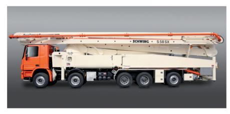
Only 48 ton gross vehicle weight make this long reach boom more versatile, faster, and it has a carrying reserve for equipment. on its 5 axles this pump is very agile on the road and on the site.
