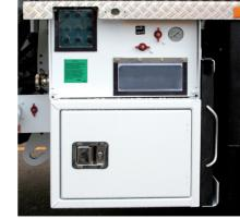
The Command centre on the ground integrates the rear panel control, chamber valve control block, the mailbox for the dockets, and a lockable equipment box.
