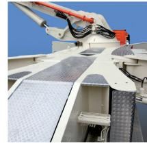
The SX outriggers leave enough space to mount a pump kit with a 2,5m stro-ke. The result is less wear and smooth pumping.
