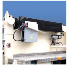
The 600 litre water tank is mounted close to the hopper and can be optionally equipped with a high pressure cleaner or a water tank heating system.
