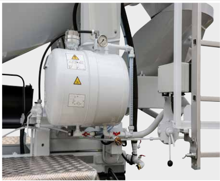
Plasticiser system 60 l (compressed air)
