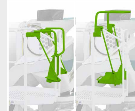
Ladder platform with step and railing elevation
