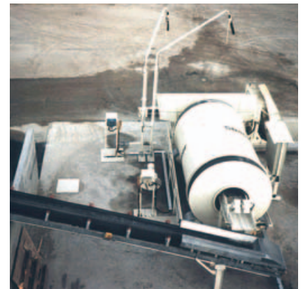
Design with conveyor belt for extracting solids.
