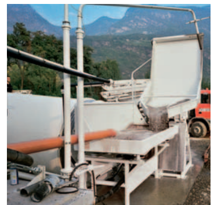
Hydraulic skip for feeding surplus materials from concrete pumps, 1,100 liter capacity.
