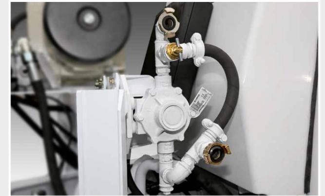
Once the concreting work is finished, the water pump facilitates cleaning of the CP 1800 D / CP 2800 D with up to 80 l/min and up to 20 bar of water pressure.
