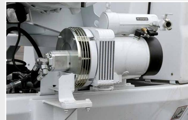
With the powerful compressor, delivery lines can be blown out with an air pressure of up to 13 bar or, for example, the coolers of the CP 1800 D / CP 2800 D can be cleaned.
