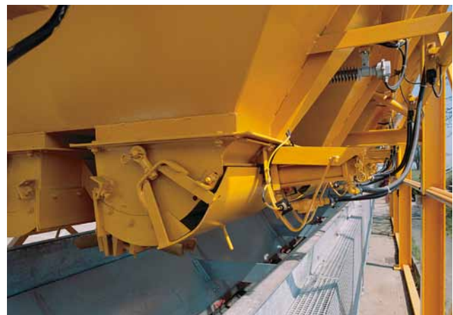
Batching gate and weighing belt for the in-line silo.
