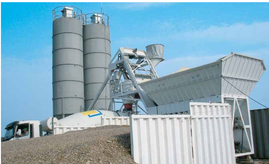
The compartment batcher with four compartments that can be fed via ramps located on both sides. The feeder skip also functions as a weighing device.
