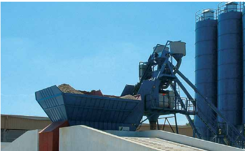
The compartment batcher with four compartments that can be fed via ramps located on both sides. The feeder skip also functions as a weighing device.
